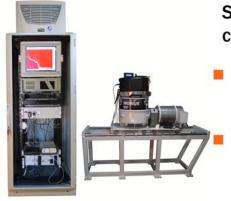
Spectrometric complex for on-line monitoring of the primary coolant «STPK-01»
